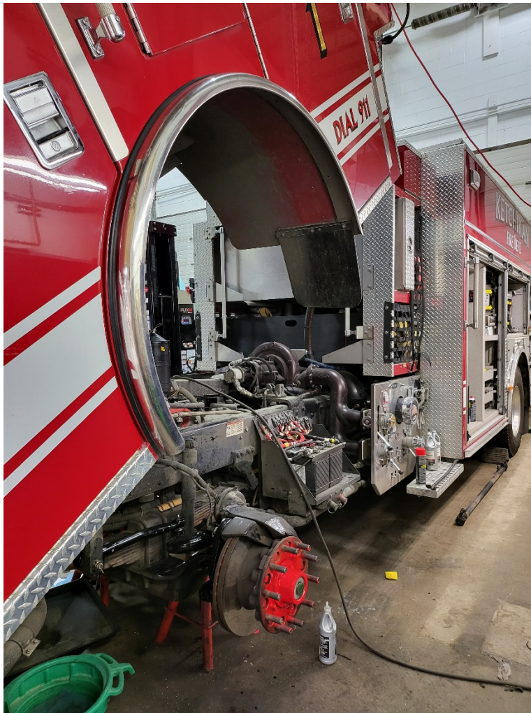
Rebuilding the Front End of Truck for KFD
